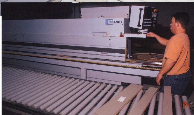
The main panel processing cell is equipped with a Holzma Optimat HPP-81 panel saw (below) and a Brandt KD-97-C edgebander (top and above) equipped with a Doucet return conveyor.
