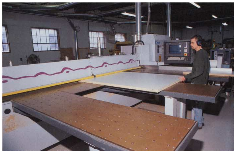
The main panel processing cell is equipped with a Holzma Optimat HPP-81 panel saw (below) and a Brandt KD-97-C edgebander (top and above) equipped with a Doucet return conveyor.
